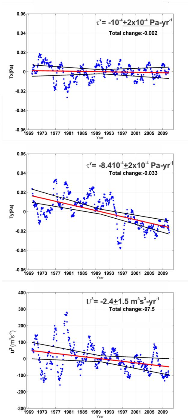
Figure 6. Long-term linear trends in monthly anomalies of the along- ( $\tau^x$ ; top panel) and cross-shore ( $\tau^y$ ; middle panel) wind stresses and wind speed cubed,  $U^3$  (bottom panel). All regressions are significant at the 95% level, except for  $\tau^x$ , which is not significant. Blue dots are the monthly anomalies after smoothing with a 13-month running mean. Anomalies have been smoothed with a 2.5-year low-pass filter.
