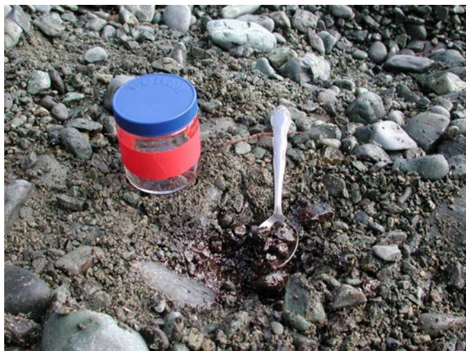
Example of I-Chem jar (4 oz.) and spoon with oiled sediments.
