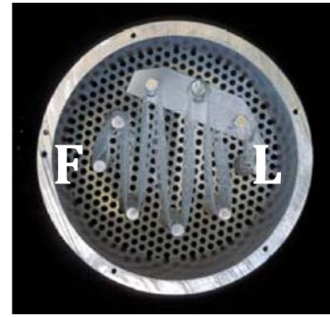
A successfully loaded puck: the first (F) and last (L) prongs are
