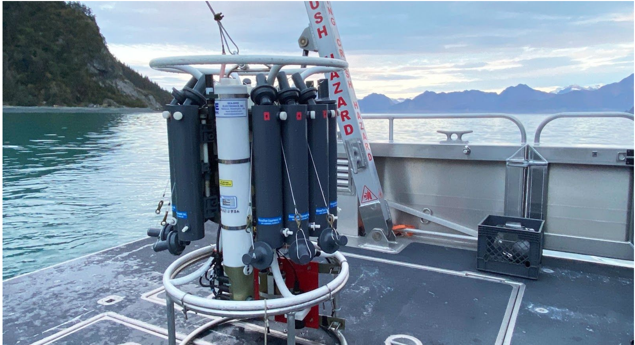
Primed and ready to grab seawater and profile the water column. University of Alaska Fairbanks Oceanographers on the R/V Nanuq prepare to deploy a rosette loaded with Niskin bottles and a CTD (conductivity, temperature, and depth) profiler near GAK1 station. Sunny Cove, Resurrection Bay, October 2020. (Photo provided by Seth Danielson.)
