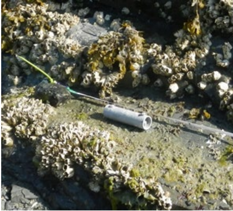
Figure 1-3. Typical installation of a HOBO temperature logger in the intertidal zone inside a PVC pipe and bolted to the substrate.
