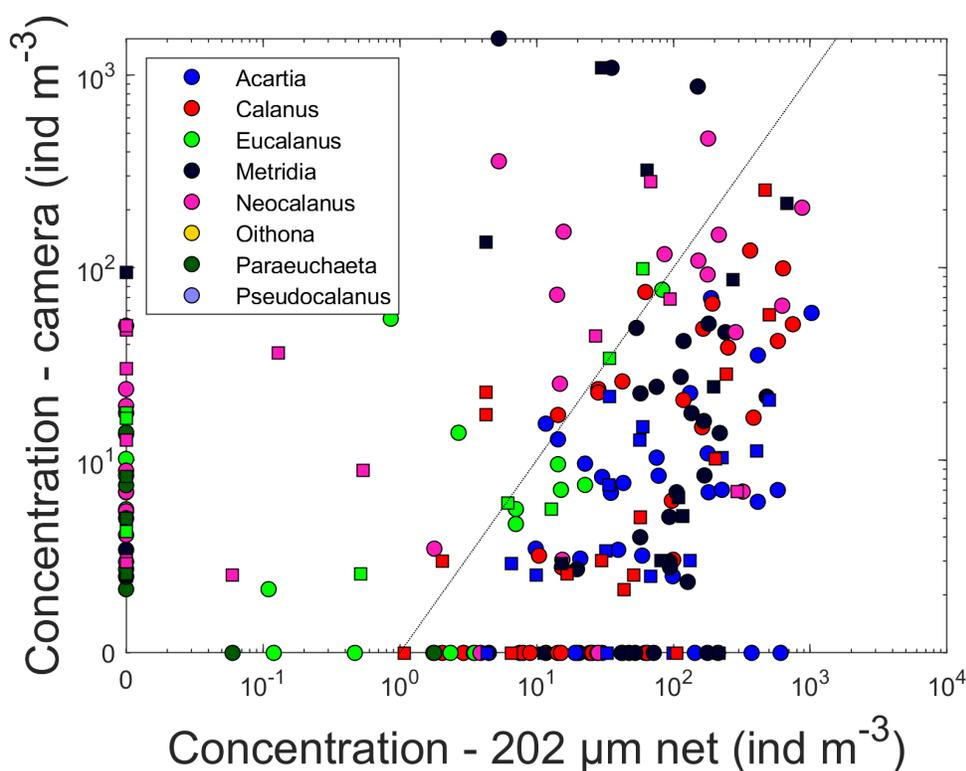
Figure 4. Comparison of abundance estimates for copepods derived from the plankton camera aboard the Prince William Sound Profiler (ordinate) and a 202  $\mu\text{m}$  plankton net. The dashed line indicates the 1:1 line. Plankton tows were done after profiler service visits, and the tow was done from 0-60 m (the depth that the profiler samples), and as close in time to a profile as possible (usually <1 hour).
