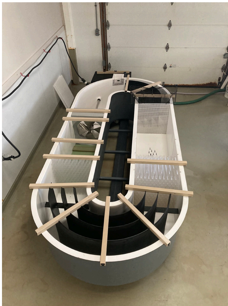
Figure 6. Photograph of the newly-constructed swim flume, including the motor (shrouded in the background), propellor, shaft, venturi, turning veins, laminizer tubes, and swim box.
